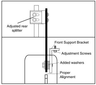
Figure 21. Proper splitter/blade alignment.
